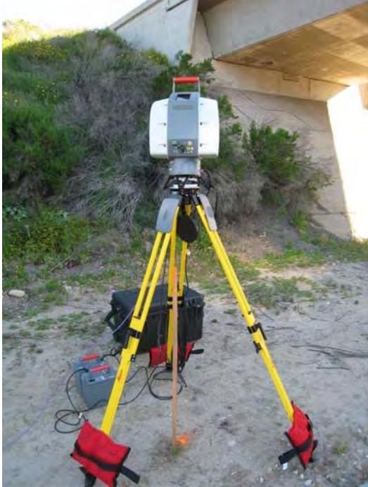
Figure 1. Leica ScanStation 2.
