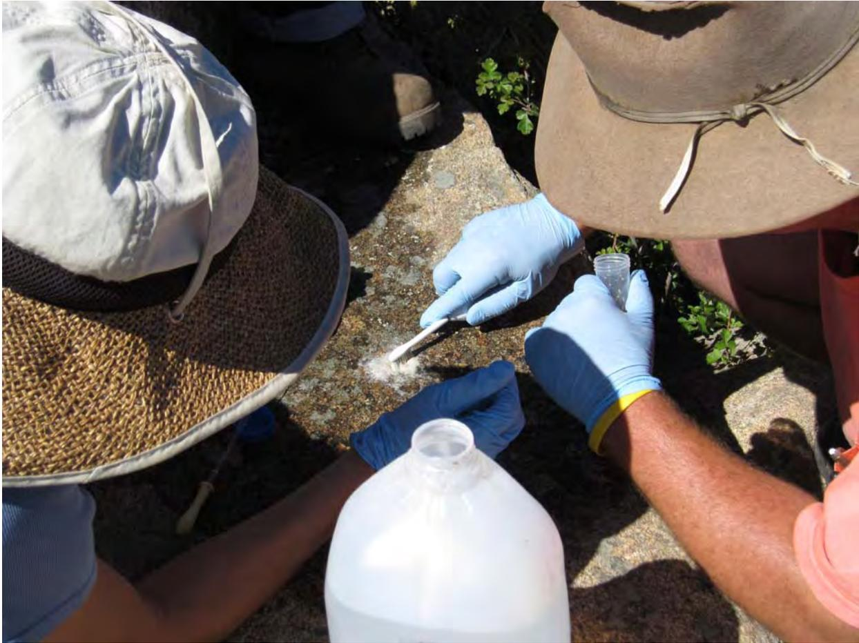
Figure 2. Scrubbing slick with sonic toothbrush and Tris/Triton and de-ionized water solution.
