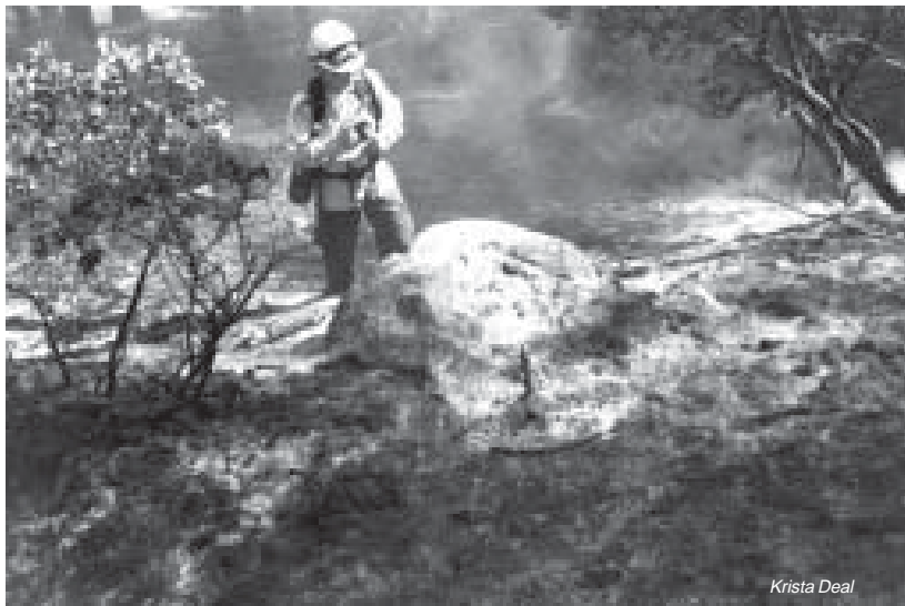
Figure 3. "BRM" boulder used in fire effects study following prescribed burn. All fuels in the immediate vicinity of the boulder were consumed. A large spall broke off the face of the boulder where the dip can be seen along the top left edge.
