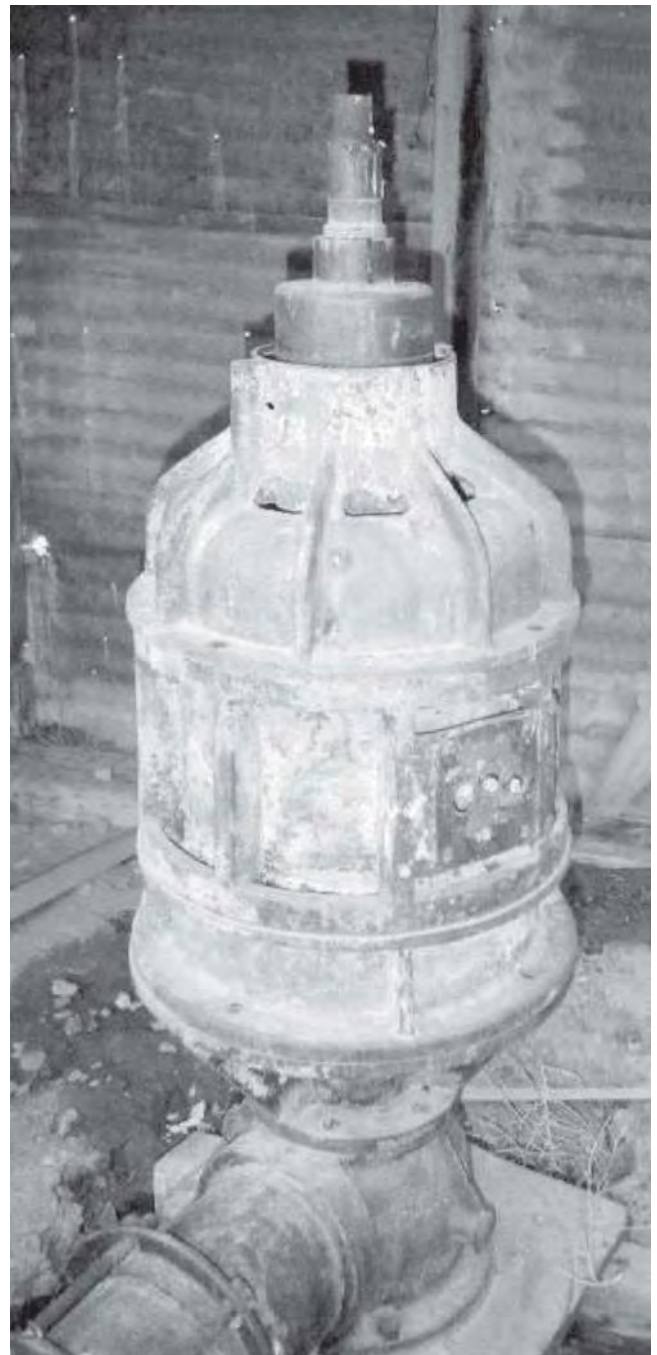
Figure 6. Electric-powered turbine pump observed in Los Angeles County; manufactured by the Peerless Company, Los Angeles, California, between 1923 and 1946.
